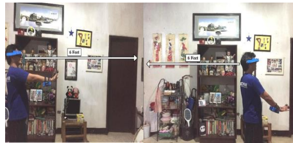
Figure 5. Maximum Reach of the Sensor for Front (Left) and Rear (Right) in the Eyeglass
